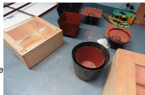
3.43 At the time of the visit it was the rainy season in Malawi and most days were overcast with little or no sun. The prototype was assembled and the functionality of the components tested. The temperature of the oil bath reached 73°C but the weather conditions prevented any further temperature rise.
