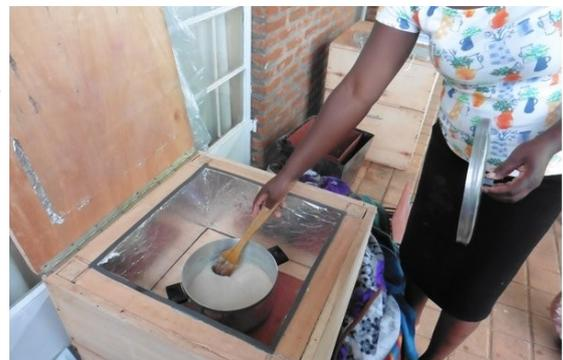
3.46 Trials were performed using the heater as a hotplate outside of the insulated cook stove. Water was heated and when at a suitable temperature a local lady used the solar powered hot plate to cook nsima porridge.
