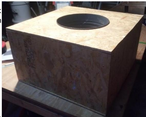
3.24 The container for the PCM needs to be robust to withstand the constant heating and cooling down and also water tight. In Malawi it is expected that these will be made by local metal workers who are experienced in making cooking pans. For the UK prototype we are using a manufactured metal waste paper bin as the container for the PCM vessel as it is our cheapest and most readily available option.
