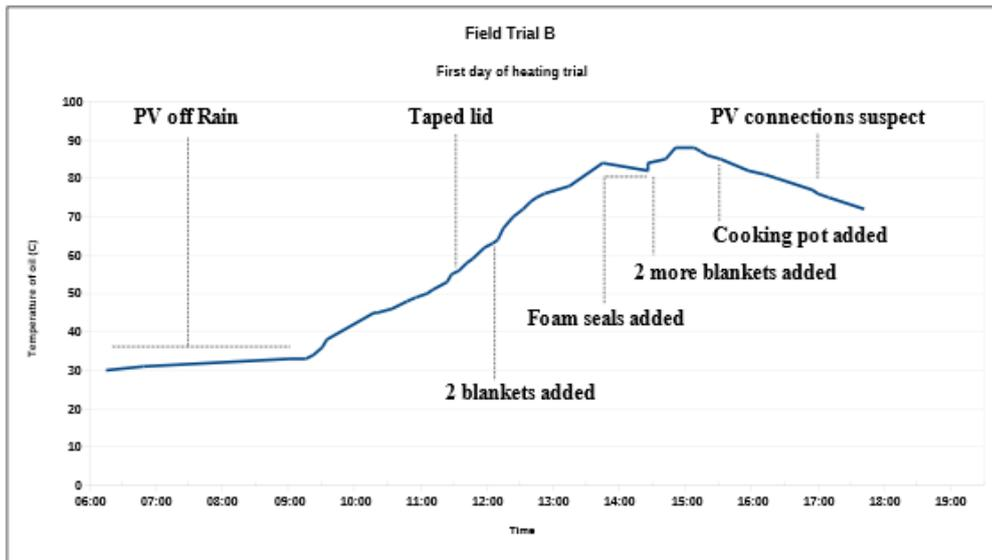
3.45 It was found that there was a large temperature differential between the oil temperature and the cooking pot temperature and it was concluded that the PCM was acting as an insulating layer. The decision was taken to transpose the oil and the PCM so that the oil was in direct contact with the heat transfer rods. This did achieve a thickened nsima paste but over too long a time to be acceptable. It also showed that the insulation was still insufficient.
